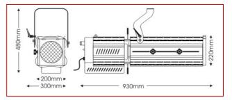
A high efficiency, powerful 200W led module featuring a PWM dimming power source harnessed in the high-specification optics of LDR profile spotlights.
